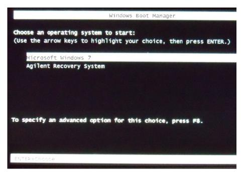
2 After a few seconds, Logic Analyzer automatically starts with the option selected in the Windows Boot Manager. Select the **Agilent Recovery system** option in the Windows Boot Manager screen using the arrow keys and then press Enter.
